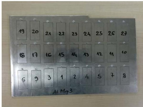
Fig. 1. Plate with specimens obtained after laser cutting,
