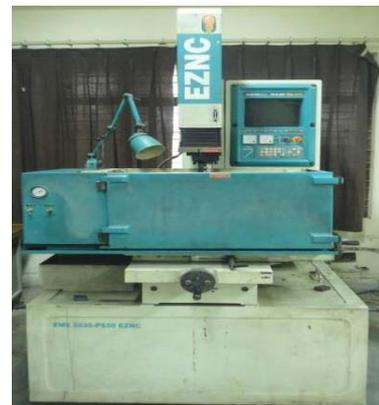
Fig.1. Physical set up of Electrical Discharge Machine
