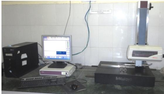
Fig.3. Mitutoyo Surface Roughness Tester SJ2100
